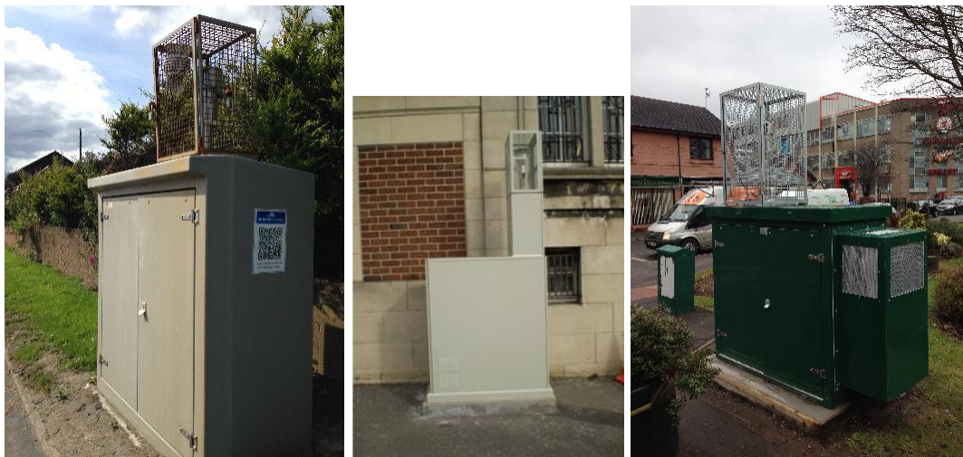
Figure 4-7: Site photos of enclosures housing a single analyser to measure PM 10 and PM 2.5
