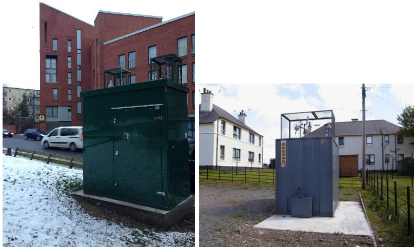
Figure 4-7: Site photos of enclosures housing a single analyser to measure PM 10 and PM 2.5
